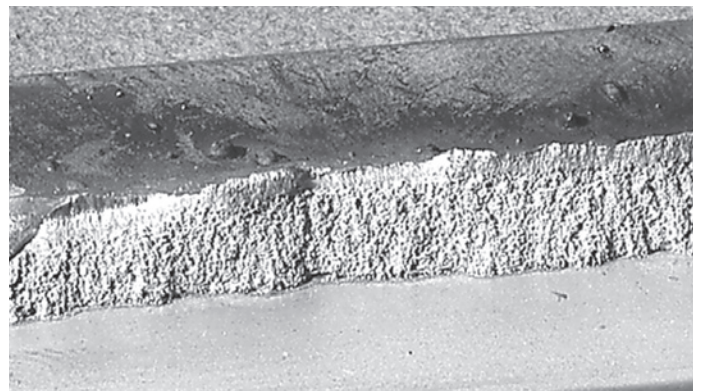
Aluminum weld with proper weld preparation shows no pores. Result - acceptable weld.
