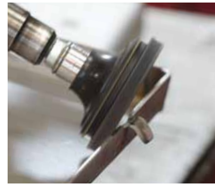
Edge chamfering a fabricated stainless component.
